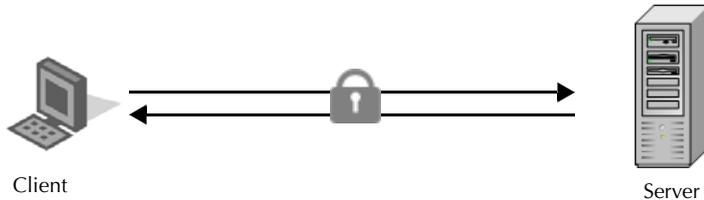
The Web Security appliance does not have access to the server's private key, so in order to inspect the traffic between the client and the server, it must intercept the connection and break the connection into two separate connections. The appliance acts as an intermediary between the client and the server pretending to be the server to the client, and the client to the server. This is sometimes referred to as being the "man in the middle."
