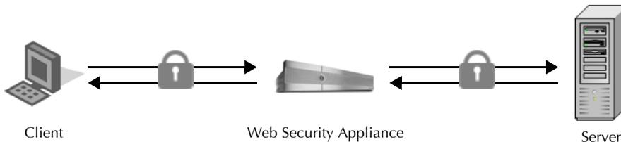
Notice that in Figure 9-4, there are two different HTTPS connections, one between the client and the appliance, and one between the appliance and the server. The appliance performs the SSL handshake twice, once with the client and again with the server:
